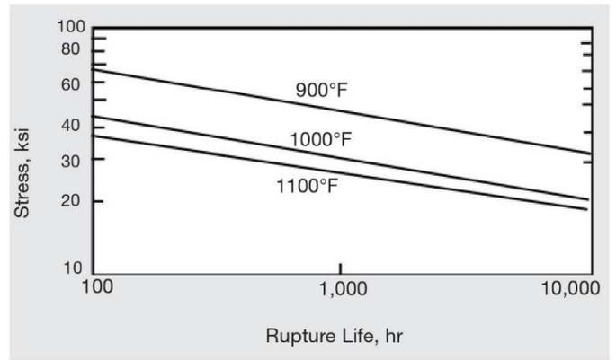
Figure 17 - Rupture life of hot-finished aged Alloy K 500
