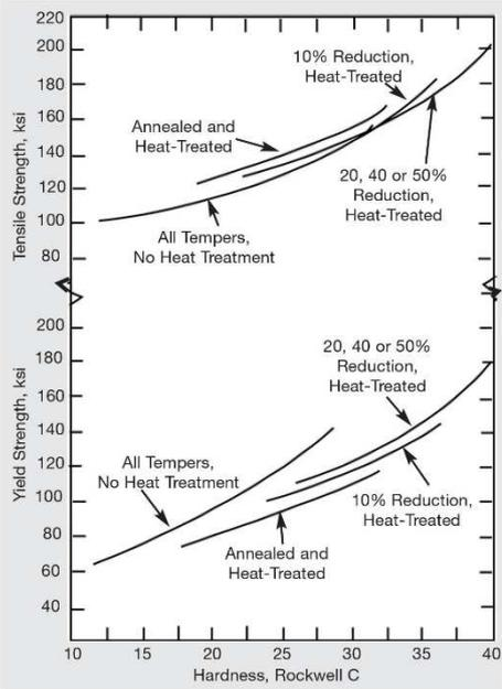
Figure 6. Approximate relationships between tensile properties and hardness of Alloy K500 strip and sheet.
