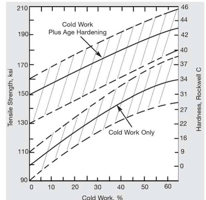
Figure 21 - Effect of cold work and age hardening on properties of Alloy K 500
