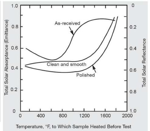
Figure 3 - Total solar absorbance at 100°F of Alloy K500 (Comparison standards; comparison pyroheliometer. Measured in air.)
