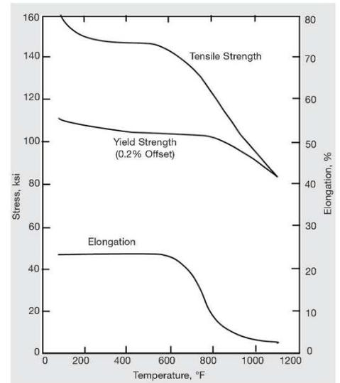
Figure 8. High-temperature tensile properties of hot-finished age-hardened Alloy K500
