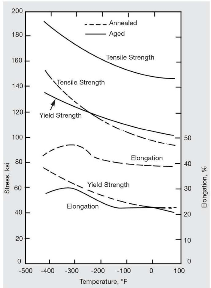
Figure 10. Low-temperature tensile properties of Alloy K500 (0.063-in. sheet).
