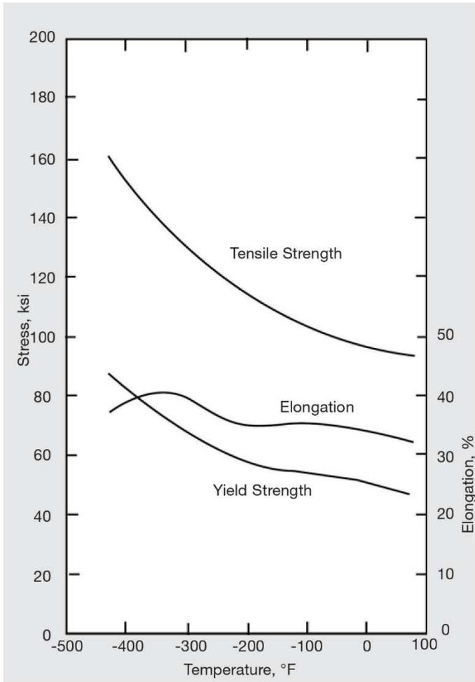
Figure 11 - Low-temperature tensile properties of Alloy K 500 welded and annealed
