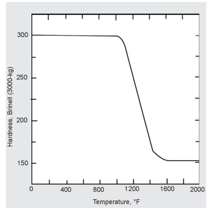
Figure 19 - Effect of water quenching from various annealing temperatures on hardness of Alloy K 500
