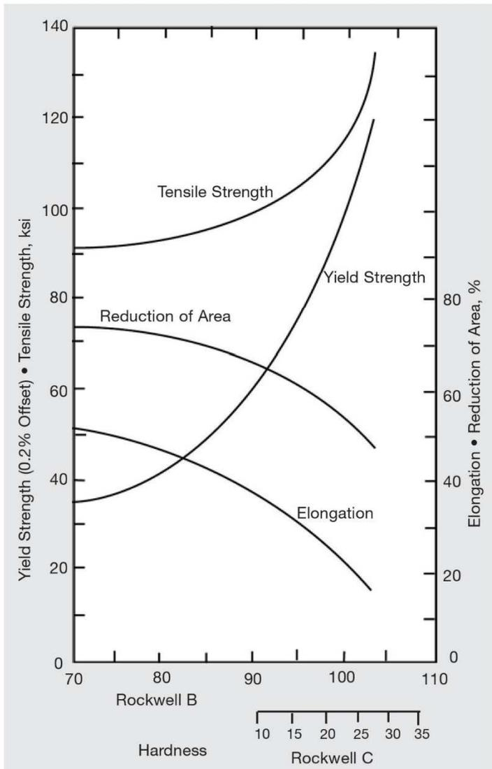
Figure 4 - Approximate relationships between tensile properties and hardness of Alloy K500 hot-finished rods and forgings and cold-drawn rods.
