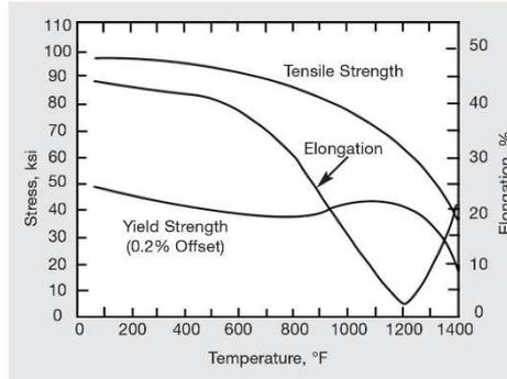
Figure 7 - High-temperature tensile properties of Alloy K500 rod (not-rolled, as-rolled).
