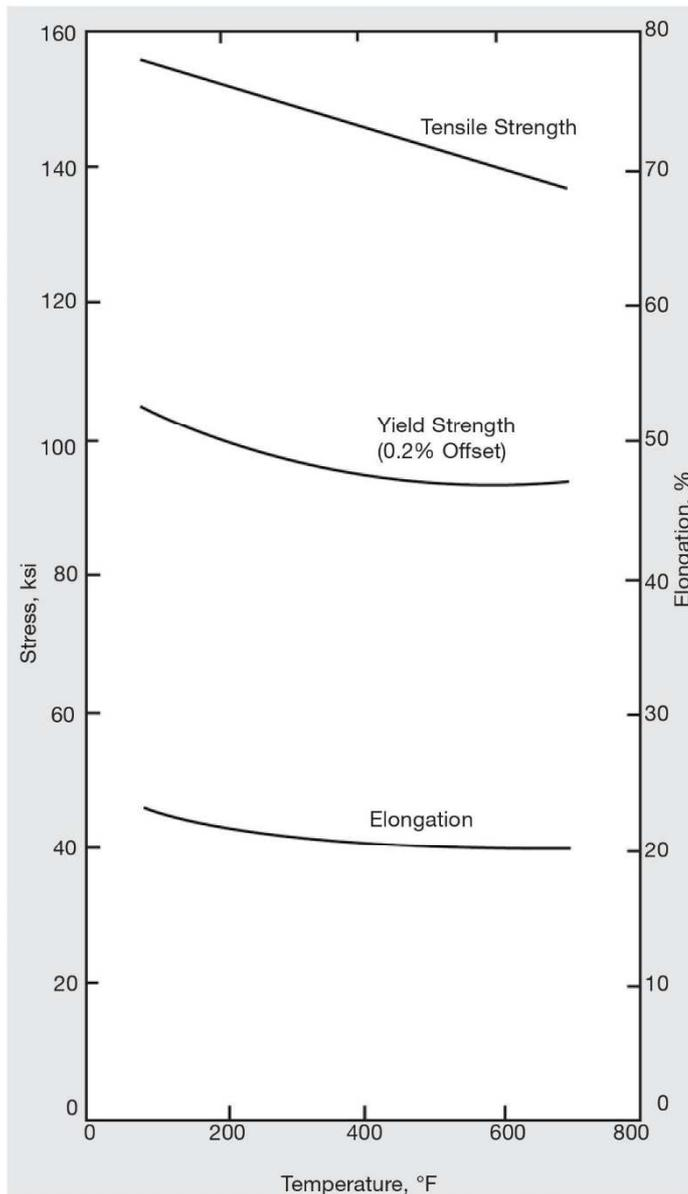
Figure 9. High-temperature tensile properties of annealed and age-hardened Alloy K500
