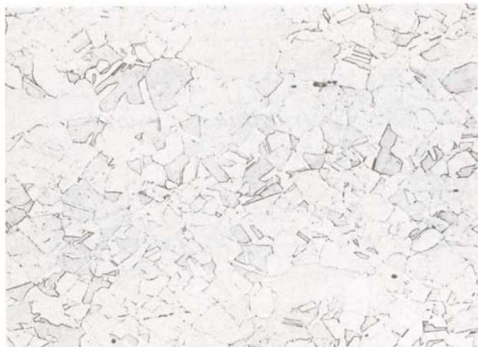
Figure 18 - Microstructure of hot-rolled, as-rolled Alloy K 500
