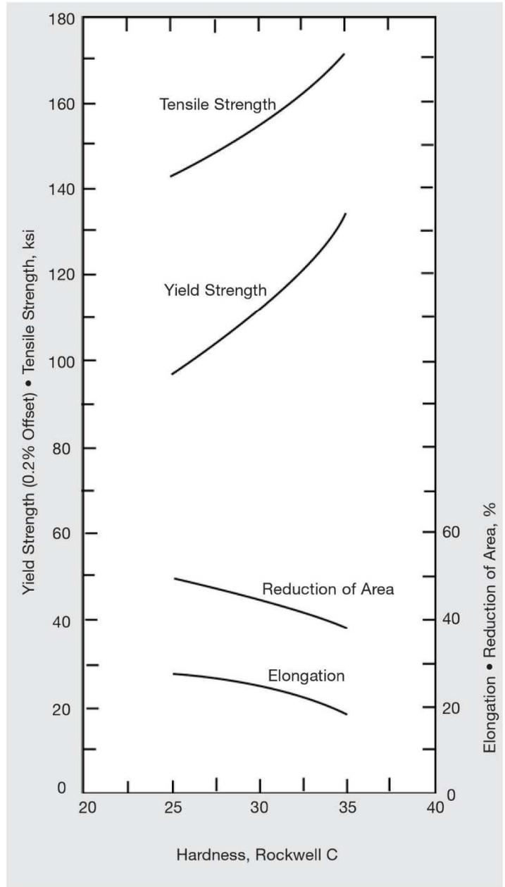
Figure 5 - Approximate relationships between tensile strength and hardness of Alloy K500 age-hardened rods and forgings.
