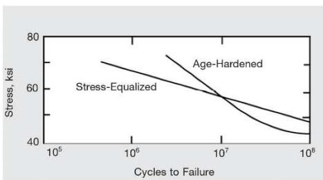
Figure 13 - Fatigue strength of commercially produced Alloy K 500 wire (0.0375-in. diameter, cold-drawn 75% after final anneal). Tested in processed condition. Data determined with a rotating-wire (5000 rpm) arc-fatigue machine.
