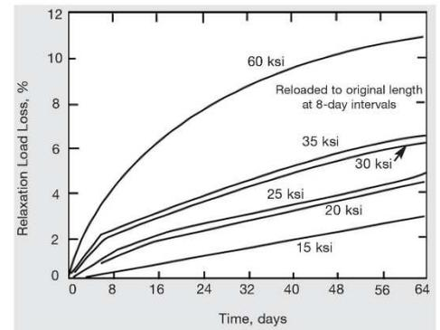
Figure 15 - Relaxation at 500°F of Alloy K 500 springs, age-hardened at 1000°F/6 hr. All stresses are shearing stresses corrected for curvature; modulus corrected for temperature.
