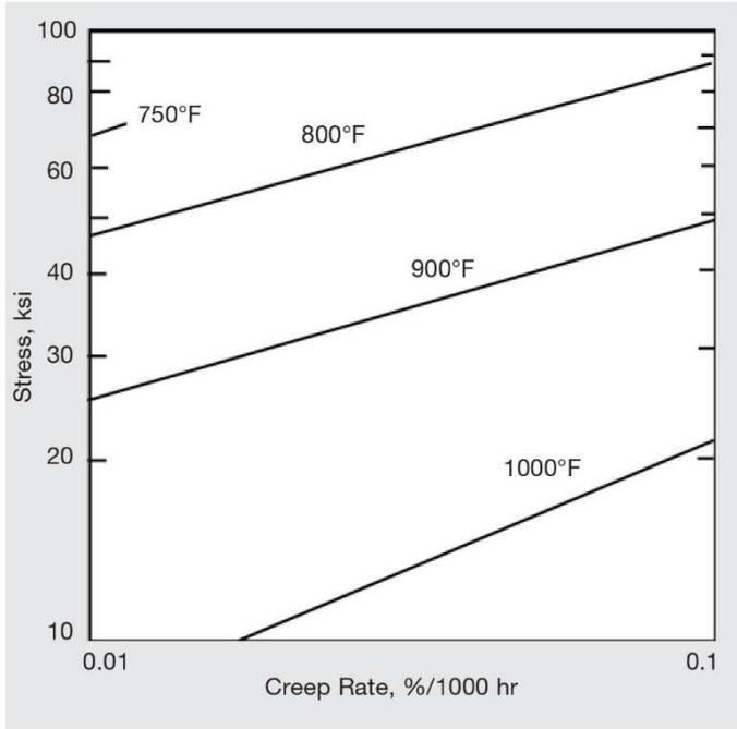
Figure 16 - Creep properties of Alloy K 500 (cold-drawnaged).
