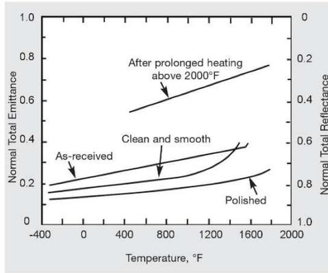
Figure 2 - Normal total emittance of Alloy K500 (Total radiation detector; comparison blackbody. Measured in a 10-micron pressure of helium.)
