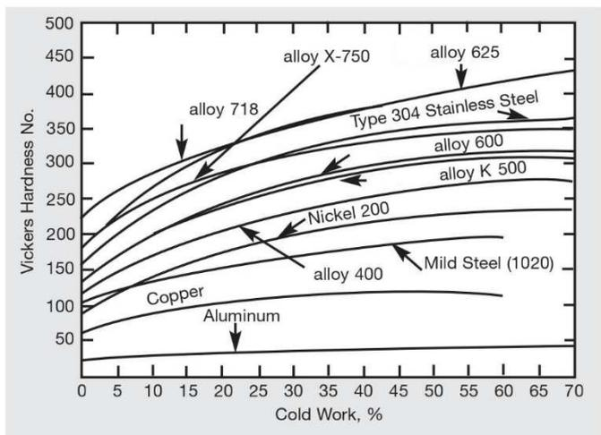
Figure 20. Effect of cold work on hardness.
