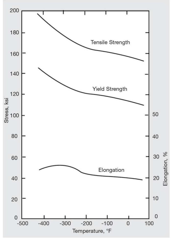
Figure 12 - Low-temperature tensile properties of Alloy K 500 welded and age-hardened
