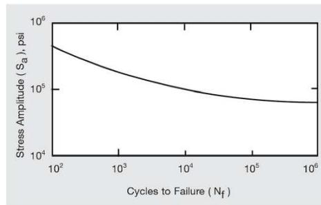
Figure 14 - Cyclic-strain fatigue of age-hardened Alloy K 500
