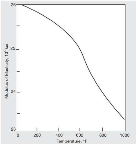
Figure 1 - Effect of temperature on modulus of elasticity in tension of Alloy K500 (determined by dynamic method).
